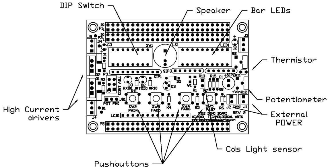
The demo program will monitor the state of the DIP switch position, the analog values of potentiometer, thermistor, and Cds light sensor as percentage of full scale. As well, the high current drivers and Bar LEDs can be controlled to be turned off or on via PC Telnet session.
