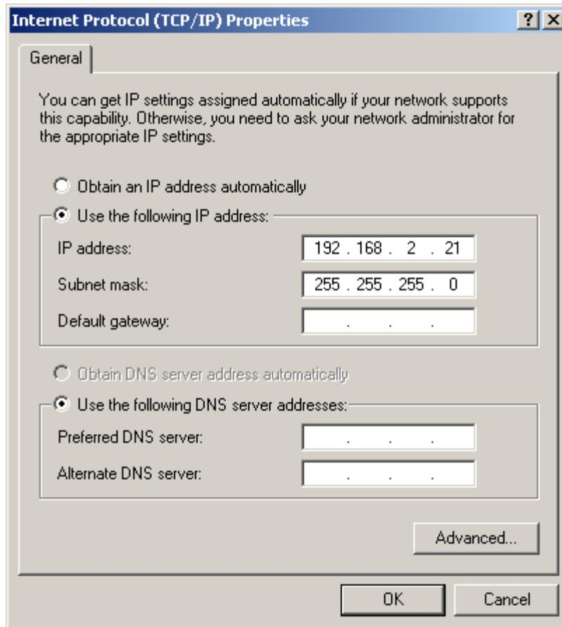
Now that the PC Ethernet Card has been configured they can now be all connected. It is better to use a HUB and a straight cable to make it easy for hardware debugging. The main reason is to be able to look at the link LED activity at a glance without having to check the back of the computer. The other reason is the Packets from the PC will be sent to all ports without them being altered and be packet sniff without difficulty.
