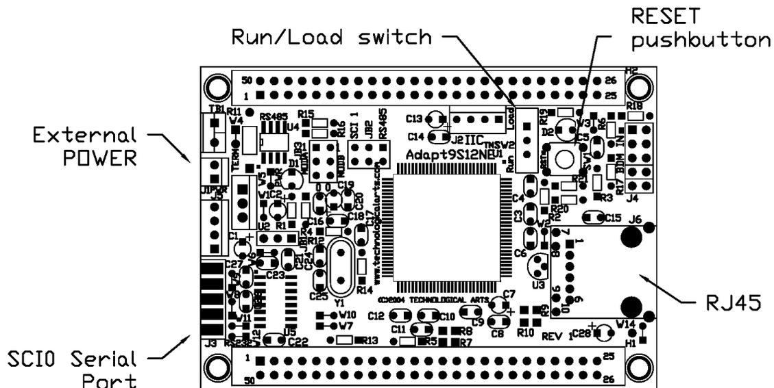
To start, slide Run/Load switch to Load, power up the board then press the RESET pushbutton momentarily. Double click on the uBUG12 icon to execute uBUG12 program. In the command bar type “con 1” (without the double quote) for COM 1 and “con 2” for COM 2. A “connect” message will appear in the uBUG12 window to indicate that PC and Adapt9S12NE64 established communications.
