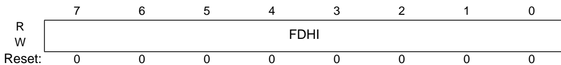
Figure 3-12 8-bit Flash Data High Register (FDATAHI)
