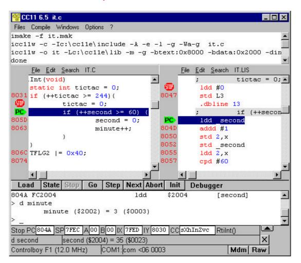
The programming interface allows you to write a program, compile it, download it, and debug it. The program can be written in assembly language, Basic, or C. The window on top is the main window. It allows you to start one or several editor windows to edit the source programs, and to press COMPILE to compile the program. You will get the output of the compilation in this window.
