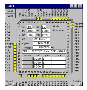
If the micro is not in the RESET state, and the speed is not at 0, you will see that the cpu runs all the time. When it does not execute an application program, it executes the talker, which is waiting for command on the serial line.
