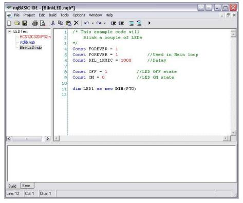
Now, let's carry on, typing in the rest of the program, starting with the delay subroutine. In the main loop there is another dropdown list to assist you.
